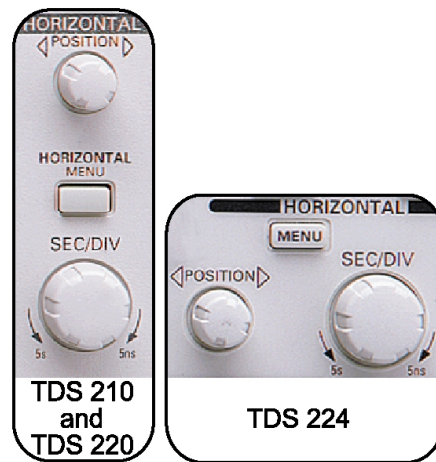
Figure 2.12: TDS200 HORIZONTAL controls
