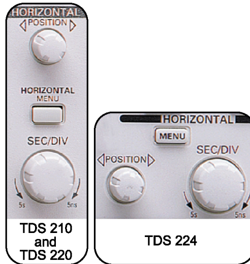
Figure 4.1: HORIZONTAL control sections
